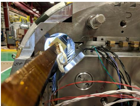
Tested in MQXFS1e magnet (VMTF stand @ IB1 TD) View of magnet RE + spliced bus
