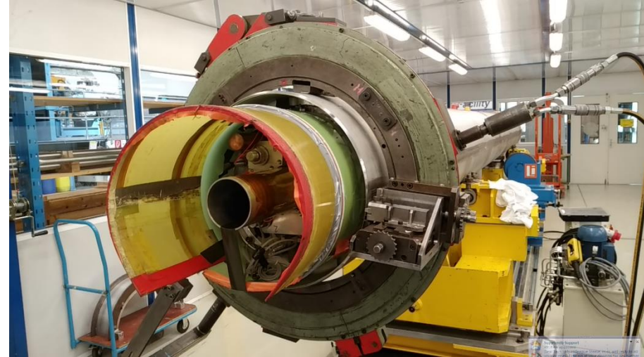
Welding preparation machining
