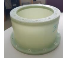
Custom made GFRE support posts in collaboration with EP-DT
