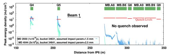
ightarrow in one case (MD2930) energy density in Q4 (Q5) 2imes(3imes) above assumed quench level, but no quench observed
