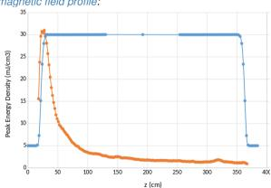
Longitudinal energy density profile in Q5 and longitudinal magnetic field profile:
