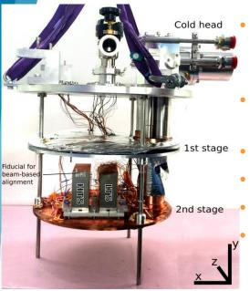
Cryocooler based cryostat to cool samples to ~4K installed in CERN's HiRadMat facility
