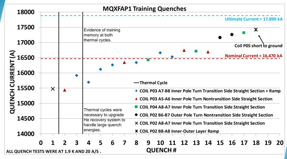
Last five quenches included CLIQ and last four did not use inner strip heaters. Testing ended after 18 training quenches due to development of short to ground.
