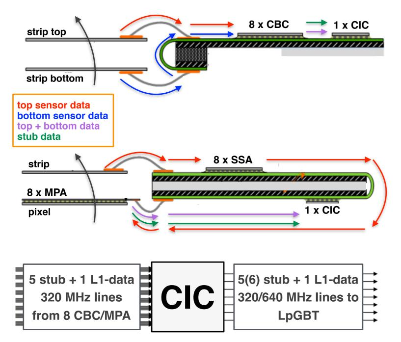
Strip-strip Module (2S) CMS Binary Chip (CBC) reads both sensor and identify stubs
