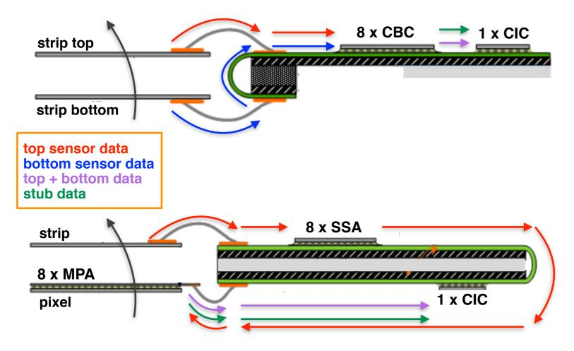
Strip-strip Module (2S) CMS Binary Chip (CBC) reads both sensor and identify stubs
