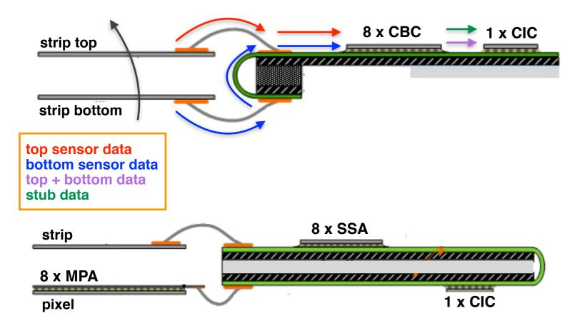
**Strip-strip Module (2S)** CMS Binary Chip (CBC) reads both sensor and identify stubs
