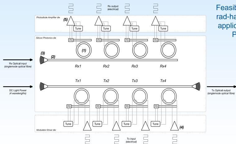
Feasibility study of a 100 Gb/s rad-hard transceiver for space applications based on Silicon Photonics micro-ring
