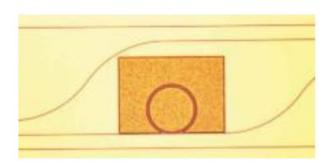
Ring radius of 50 μm => C ~0.08 pF Energy/bit ~ 0.7 pJ/bit
