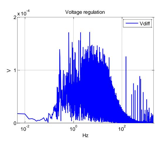
The spectrum of Vdiff, with no control of the current, is only affected by the flux jumps (apart of the harmonics of the converter)
