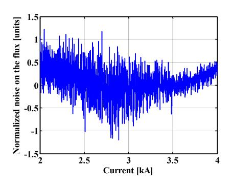
We analyze the residuals from a linear fit: we see a "noise" on the measured flux with relative amplitude up to 1\*10<sup>-4</sup>
