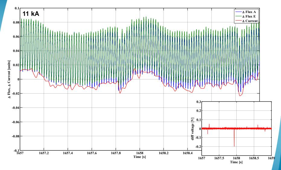
At higher field we see a perfect agreement (<10-6) of fluxes and current. The state of the flux we see the noise at 50 Hz that is filtered on the current.
