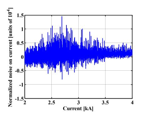
We analyze the residuals from a linear fit: we see a "noise" on the measured current with relative amplitude up to 1\*10<sup>-4</sup>
