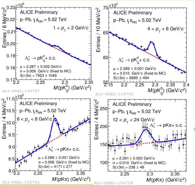
Signal extracted via an 0 invariant-mass analysis.
