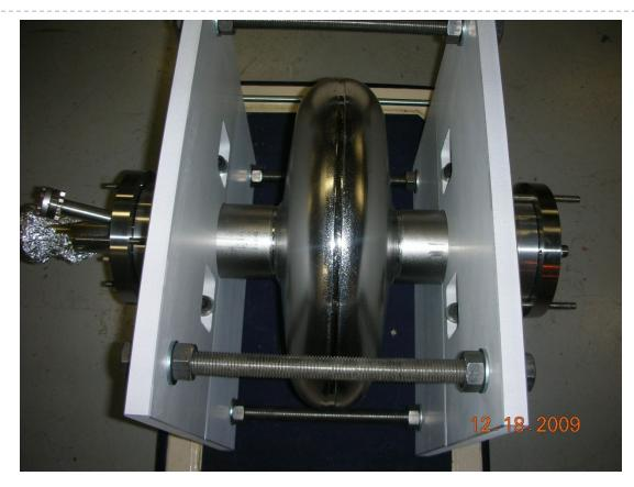
704 MHz monocell cavity (β = 0.5) manufactured by CEA/Saclay and available at CERN for validating surface preparation procedures and test equipment
