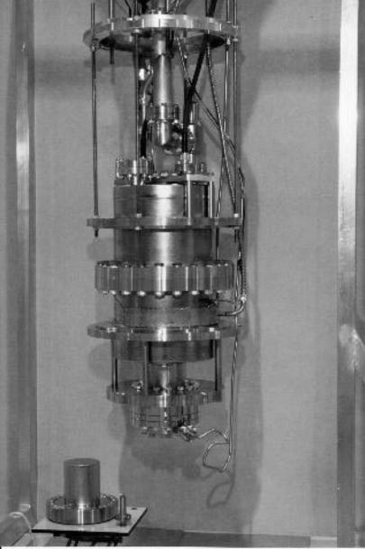
Quadrupole resonator for testing SRF samples at 400, 800, 1200, ... MHz
