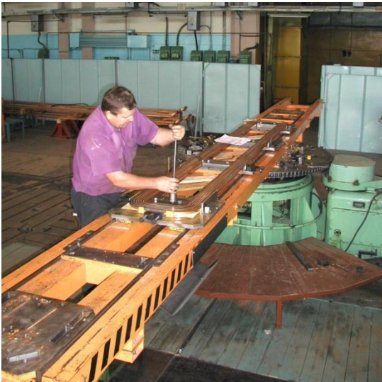
Dipoles racetrack coil
