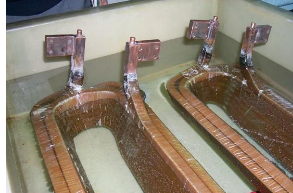
coil electrical test (under water !)
