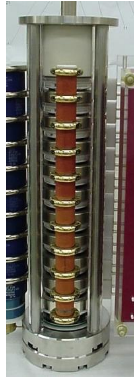
Stack of high-power semiconductor switches (GTOs)
