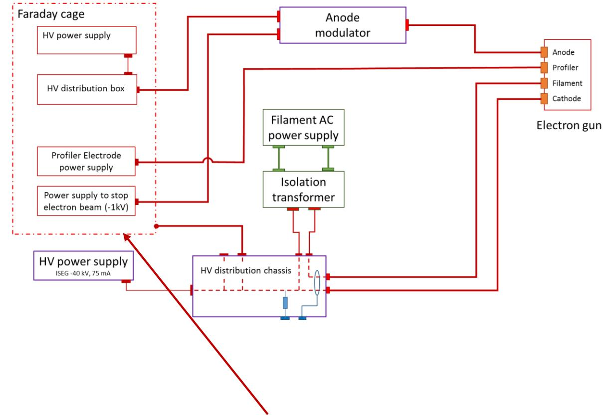
Extraction voltage is up to **40 kV**
