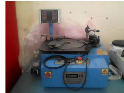
Mechanical polishing for substrate before chemical preparation/cleaning
