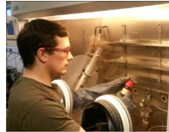
Glove box Facility to handle safely CVD/ALD Precursor chemical
