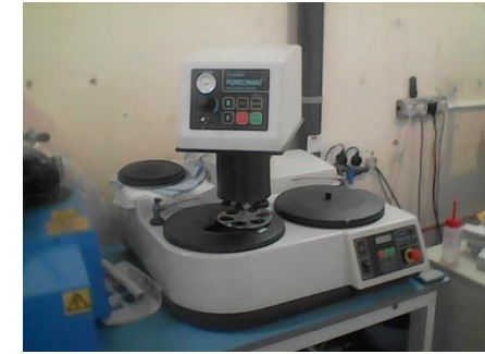
Mechanical polishing for substrate before chemical preparation/cleaning
