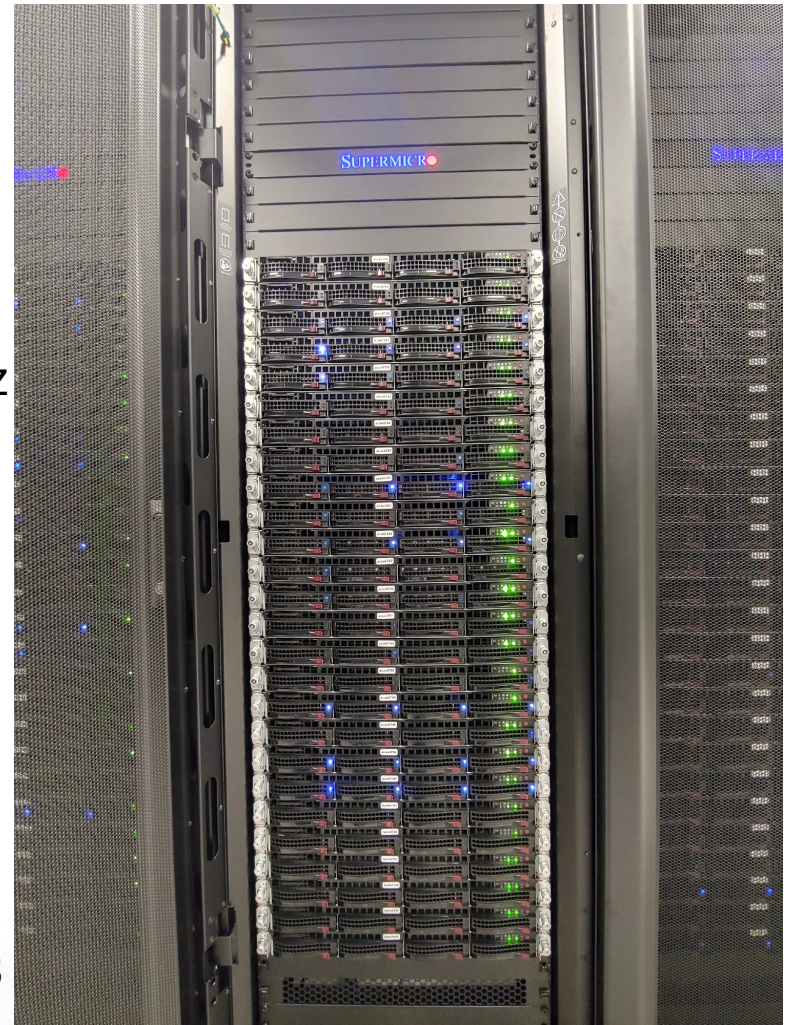
Rack of New EPYC-based Supermicro 1023US-TR4 Servers
