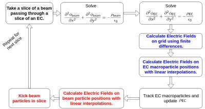
Beams are sliced in  $\zeta = s \frac{\beta}{\beta_0} - \beta ct$ . From the point of view of the EC, *s* does not change and  $\zeta$  is basically **time!** We propose to modify the kicks to the beam particles to support long-term tracking.
