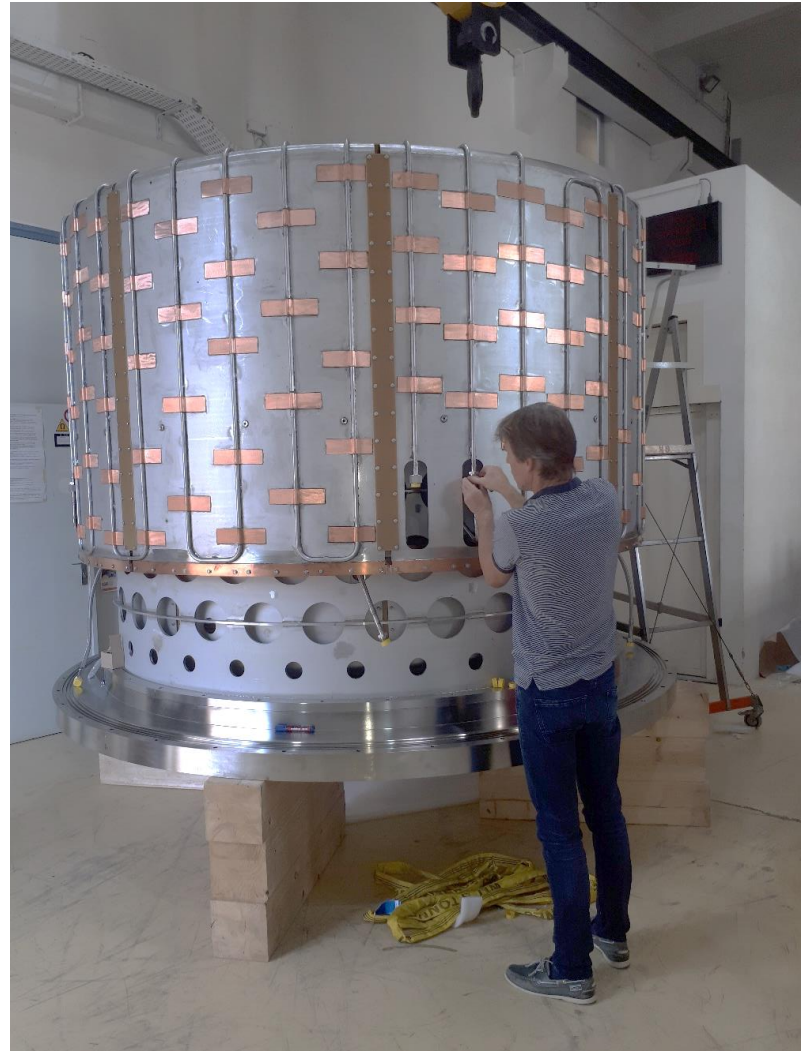
Dummy assembly of the cryostat
