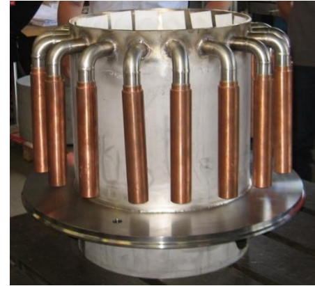
Cold fingers (i.e. 1.75 - 1.8 K heat exchanger)
