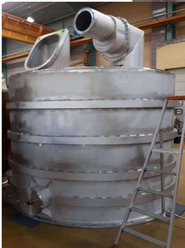
Outer vacuum chamber (on top plate : cryo line and quench line connections)
