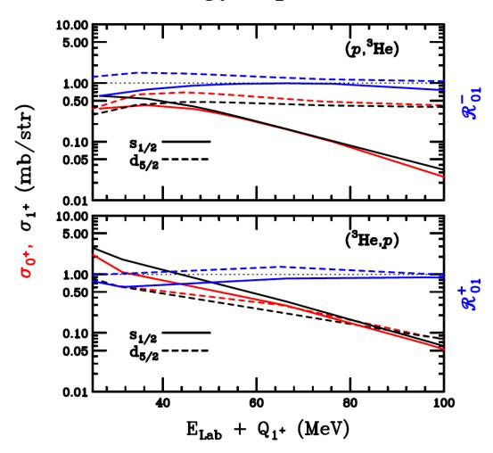
np WU's as a function of the bombarding energy plus the Q-value to the 1<sup>+</sup>state, for the representative cases of the  $s_{1/2}$  and  $d_{5/2}$  orbits.
