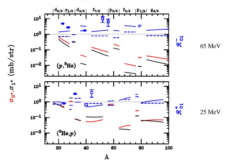
Second-order DWBA calculations with the code FRESCO, with conditions relevant to the filling of the different (n, j, l) orbits at the N=Z line, from  $^{16}$ O to  $^{100}$ Sn.
