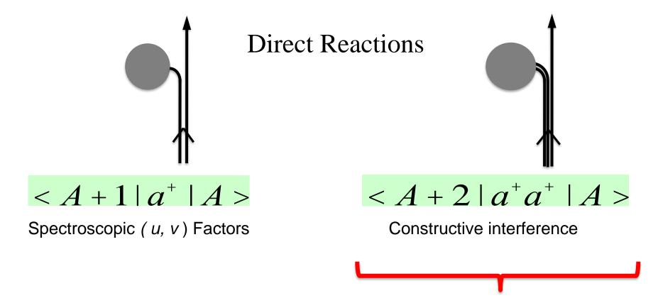
Two particle transfer reactions like (t,p) or (p,t), where 2 nucleons are deposited or picked up at the same point in space provide an specific tool to probe the amplitude of this collective motion.
