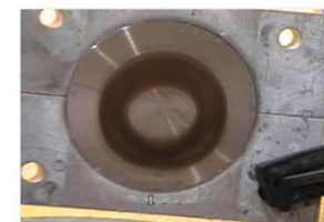
10g Th target irradiated at IPF in support of preliminary 225 Ac/ 213 Bi generator evaluation studies. Note the uniform, rastered beam pattern in the exit window.
