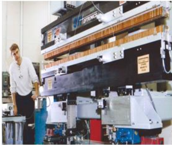
A view of the APS INSERTION DEVICE
