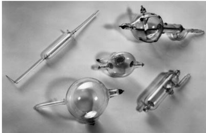
Crooke tubes used at the end of the 19th century to study electric discharges in gaseous media
