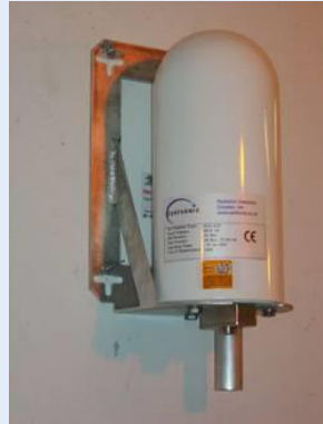
Gas filled, high pressure ionization chamber
