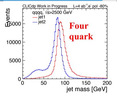
Four quark sample has narrow peaks around W and Z masses → sizeable tails to higher masses
