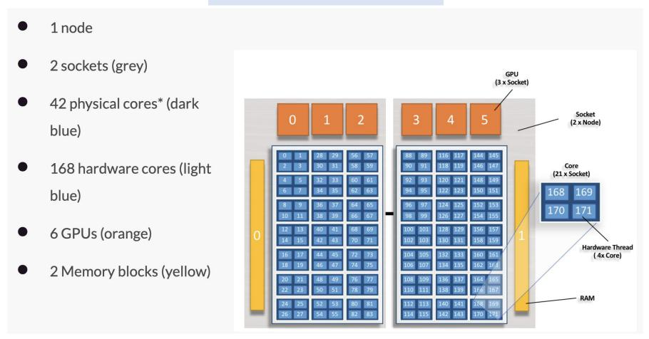
jsrun utility allows for fine grained allocation of CPU and GPU per MPI rank, as well as choice of SMT level. Large parameter space!
