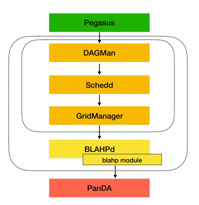
The object of the Grid ASCII Helper Protocol (GAHP) is to allow the use of the client library or package of a grid or cloud service via a simple ASCII-based protocol. A process which implements GAHP is referred to as a GAHP server. GAHP is designed to handle both synchronous (blocking) and asynchronous (non-blocking) calls.
