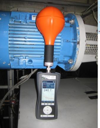
Left: Stray field of asynchronous motor fed by a VSD
