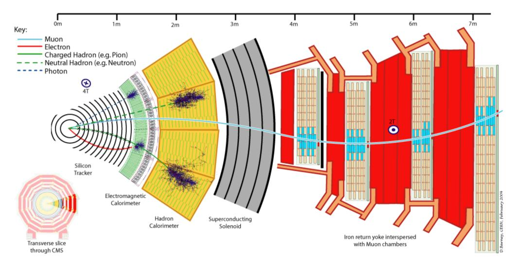
Particles leave hints of their passage in sub-detectors. Specific (but overlapping) pattern for each particle type.
