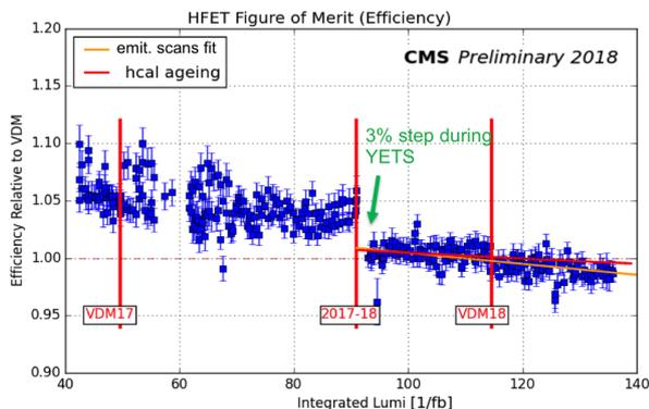
Figure 2: HFET algorithm efficiency in 2017–2018 defined from emittance scans with respect to the vdM calibration fill in 2018.
