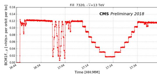
Figure 1: The hit rate reported by BCM1F pCVD during emittance scans in X and Y planes (17:00–17:05) and a  $\mu$  scan (17:10–17:30). Three smaller drops in rate correspond to the LHC beam optimizations, which took place just at the beginning of stable beams, before and after the  $\mu$  scan.
