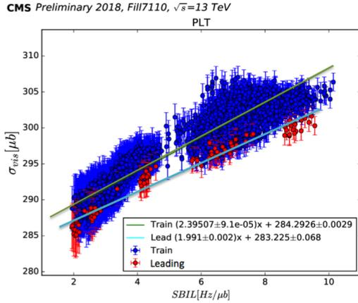
Figure 4: PLT  $\sigma_{vis}$  as a function of single bunch instantaneous luminosity in Fill 7110 for leading and train bunches with first-order polynomial fits.
