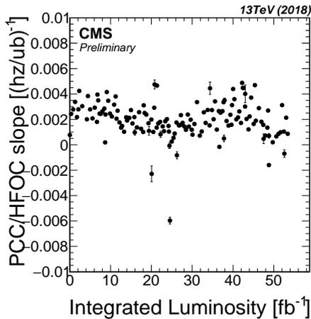
Figure 8: Results of the linearity studies for all 2018 fills for PCC and HFOC. Each point represents the slope of the first-order polynomial fit to luminosity ratios per fill as a function of integrated luminosity [3].
