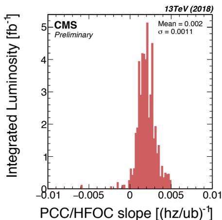
Figure 9: The slopes measured from the first-order polynomial fit to luminosity ratios PCC/HFOC per fill binned and weighted according to the luminosity in that fill [3]. Histogram of Fig. 8.
