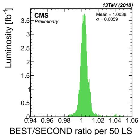
Figure 7: Histogram of luminosity ratio values between the best and second-best luminometer, weighted by luminosity. The standard deviation of the histogram is taken as the resulting systematic uncertainty [3].
