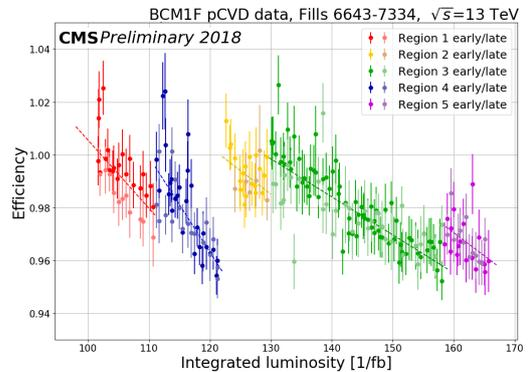
Figure 3: BCM1F pCVD efficiency in 2018 pp data-taking period defined from emittance scans with respect to 2018 vdM calibration fill.
