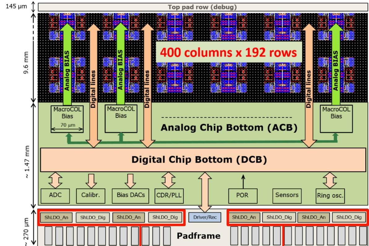
Shunt-LDO components on chip bottom
