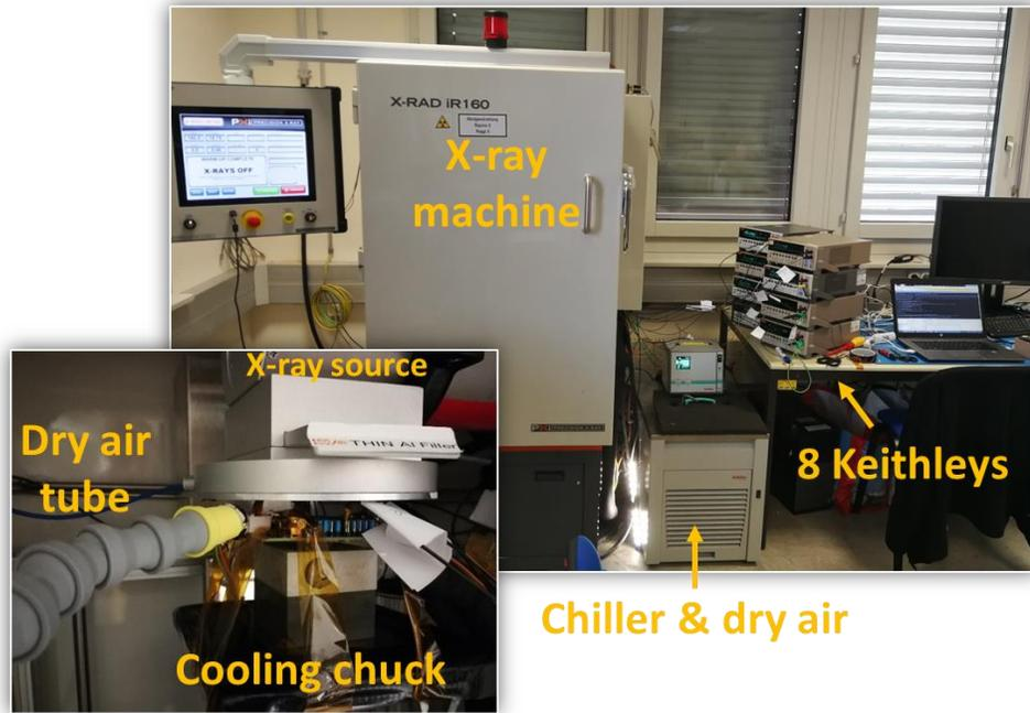
Shunt-LDO is fully functional after 600Mrad at 0C:
