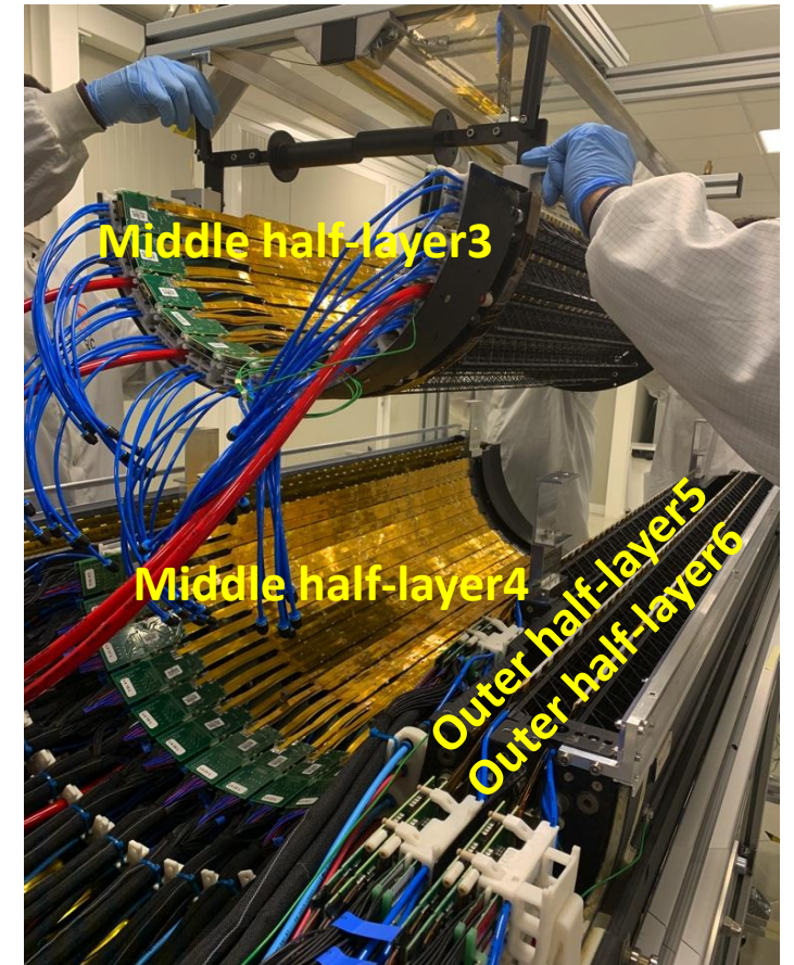
Outer barrel assembly completed
