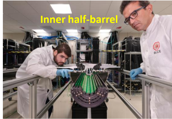
Inner Barrel assembly completed: fully functional
