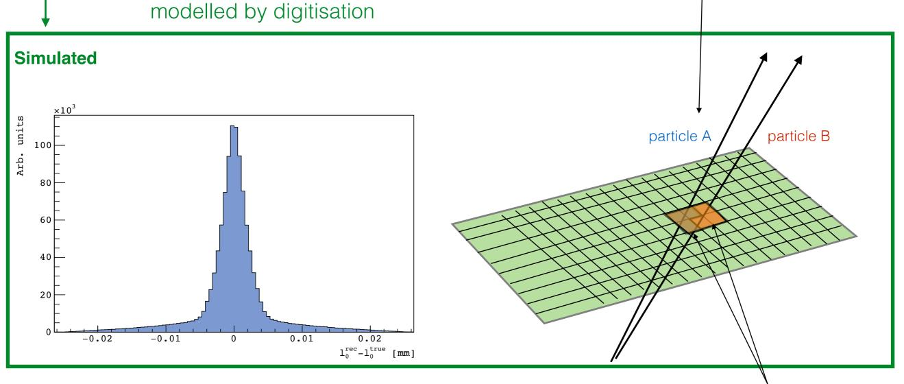
2 measurements simulated + merged into 1 measurement
