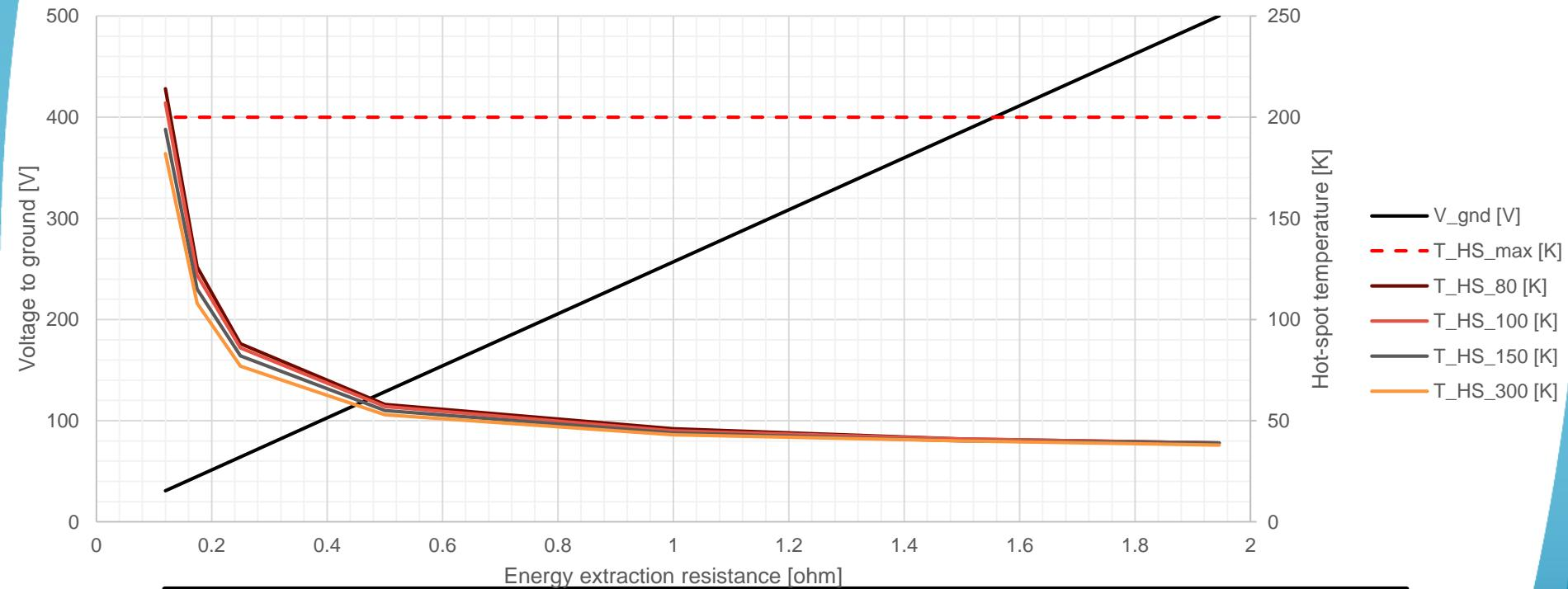
With the maximum temperature (**200 K**) and voltage to ground (**500 V**) the permissible energy extraction resistance values span from **0.12** to **1.9 Ω**.
