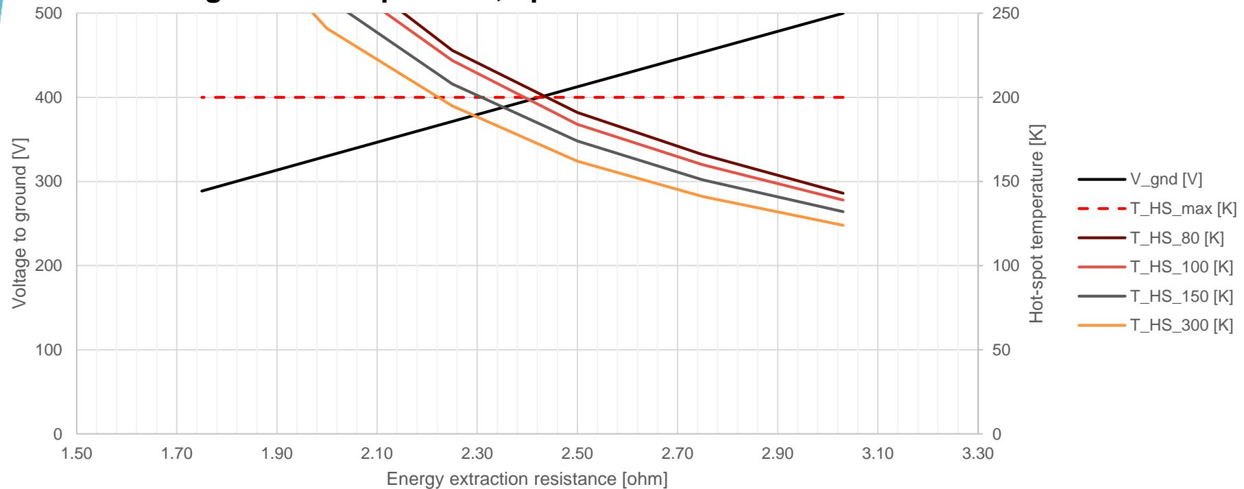
With the maximum temperature (**200 K**) and voltage to ground (**500 V**) the permissible energy extraction resistance values span from **2.46** to **3 Ω**.
