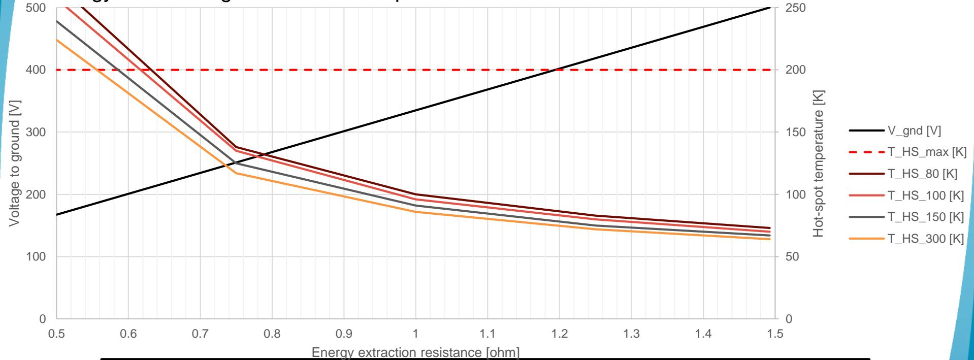
With the maximum temperature (**200 K**) and voltage to ground (**500 V**)
