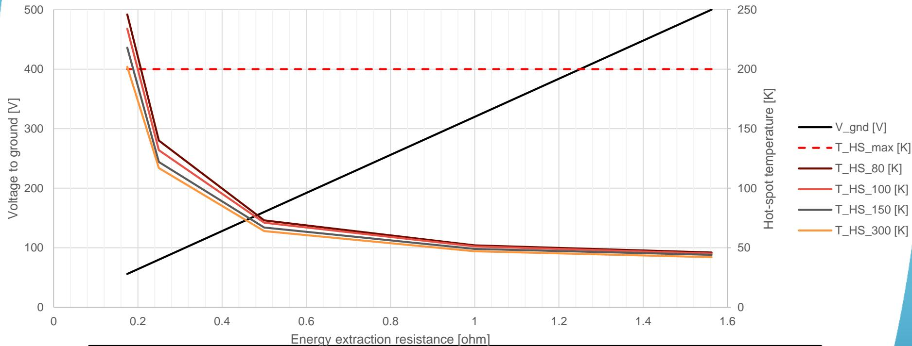
With the maximum temperature (**200 K**) and voltage to ground (**500 V**)
