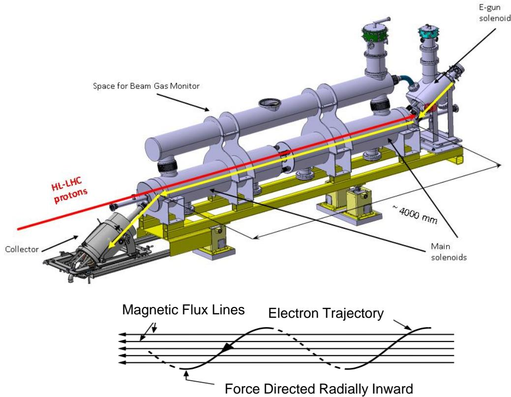
The Hollow Electron Lens system consists of multiple superconducting magnets for
