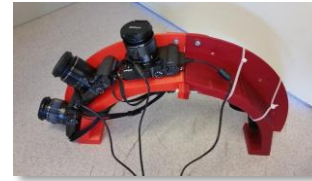
HD camera system for tunnel dome view
