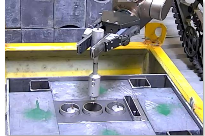
Radioactive sample handled by a robot
