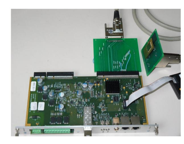
• Example: The Pixel chip and SRS integration - complete system
