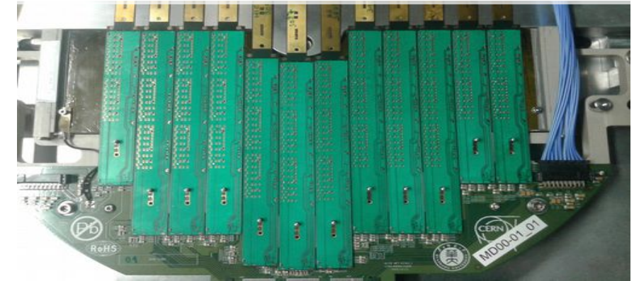
Disk fully equipped with ladders
