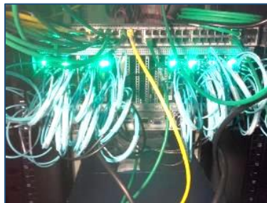
Event builder: Vertical slice setup already cabled with fibres and operational
