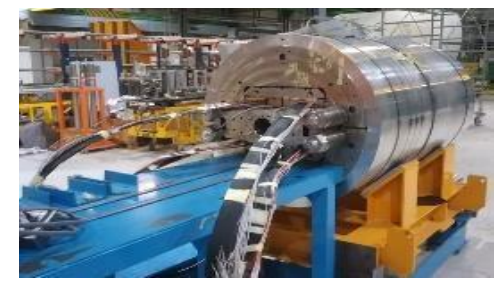
2018: FRESKA2 (100 mm aperture, 14.6/14.95 T bore/peak at 12.1 kA, 1.9 K)
