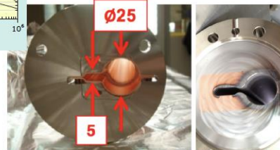
MAX IV vacuum chamber: before and after NEG coating
