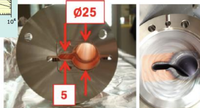
MAX IV vacuum chamber: before and after NEG coating
