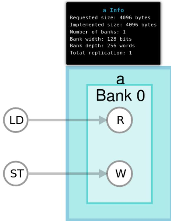
*You can see here that we are no longer separating the memory into banks but instead coalescing 4 access in to a wider 128 bit access.*
