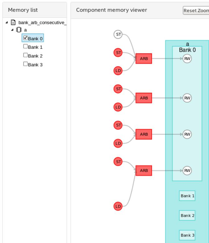
*Here again you see the 9 access aggregating on the 4 ports with the 8 simultaneous accesses being storable.*
