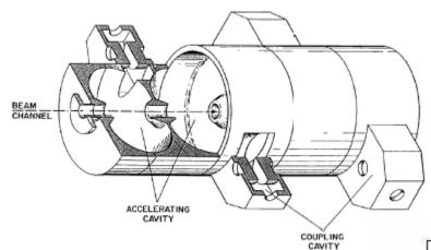
Chain of cells, coupled via slots and off-axis coupling cells. Invented at Los Alamos in the 60's. Operates in the  $\pi/2$  mode (stability).
