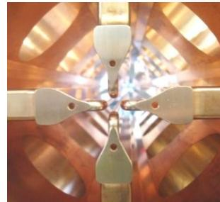
Beam goes into the paper in between the 4 vanetips 10/4/2019 19
