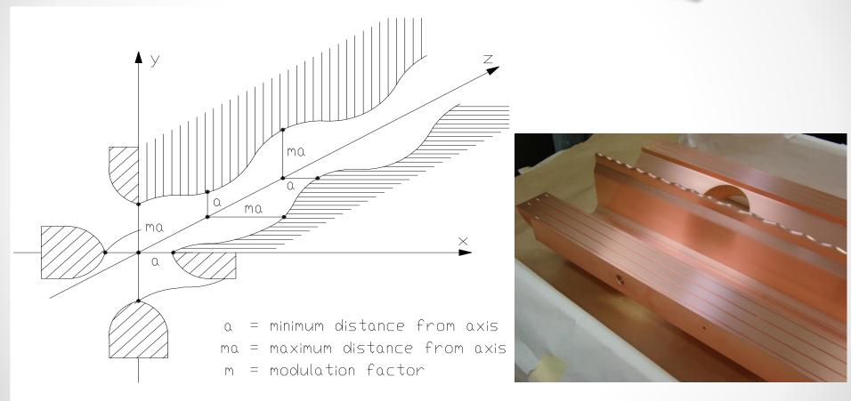
longitudinal modulation on the electrodes creates a longitudinal component in the TE mode
