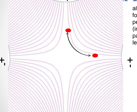
alternating gradient focussing structure with period length  $\beta\lambda$  (in half RF period the particles have travelled a length  $\beta\lambda/2$ )
