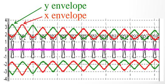
sequence of focusing and defocusing quadrupoles
