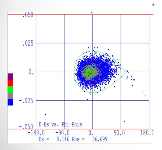
it's the (possibly fictitious) particle that we use to calculate and determine the phase along the accelerator. It is the particle whose velocity is used to determine the synchronicity with the electric field. Design for that particle and provide longitudinal focusing so that the other stick with it!
