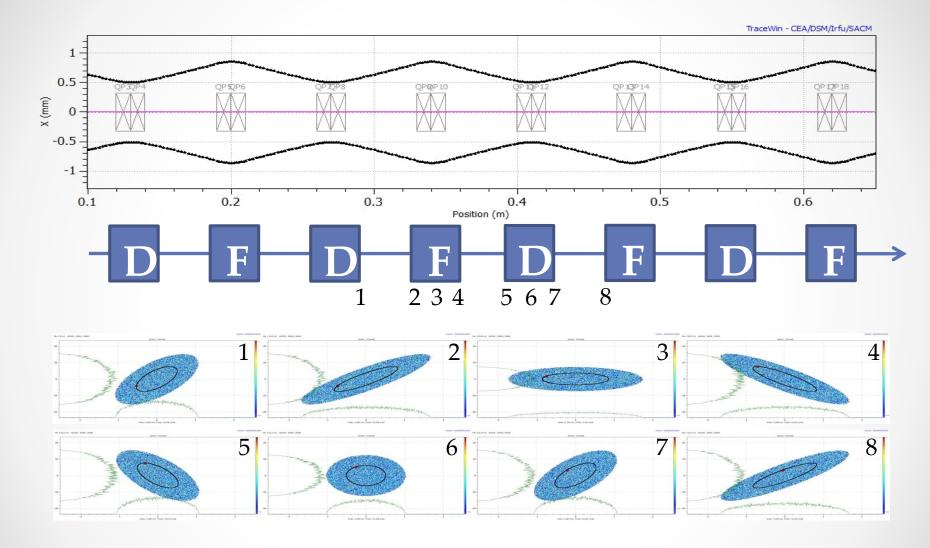
The beam is matched, after every period, the twiss parameters are identical.
