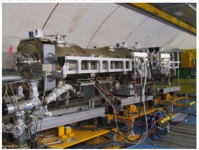
TPSG and MSE (magnetic septum) installed at HIRADMAT irradiation test facility in 2012: impacted with LHC nominal intensity (288b and 1.1 × 10<sup>11</sup> p/b): both devices survived!
