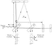
A: light source; B: partially silvered glass plate; C and E: mirrors; D and F: superimposed light beams
