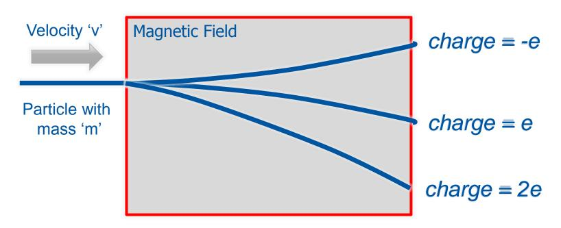
The larger the energy of the beam the larger the radius of curvature
