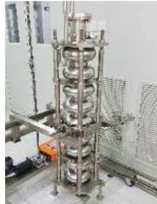
2 bare cavities (LG): Q_0 \sim 1.8 \times 10^{10} @ 16MV/m, E_{\max} \sim 26 MV/m
