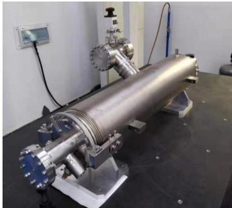
4 dressed cavities (FG): Q_0 \sim 2 \times 10^{10} @ 16MV/m, E_{\max} \sim 25 MV/m
