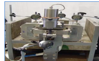
Lever Tuner – Testing and qualification up to LN2)
