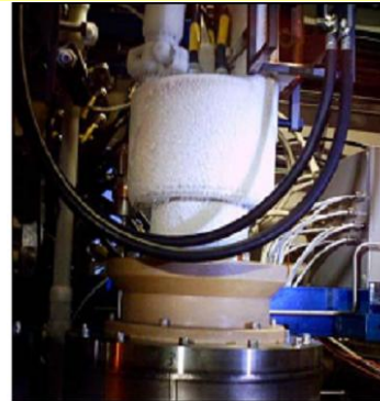
Determination of excessive frosting in cryogenic subsystem & re-evaluation of safety valve size etc.
