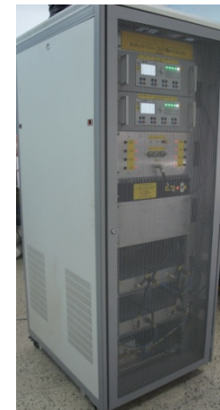
20kW wide band SSPA delivered to CERN
