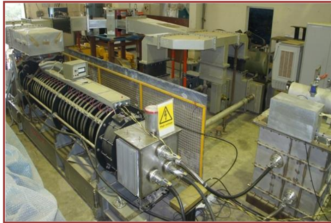
CERN klystron and circulator tested at 1MW peak power at RRCAT test stand.
