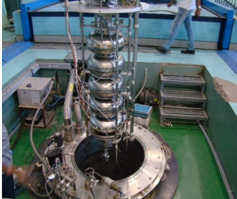
Lowering in VTS cryostat
