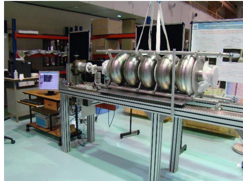
Inspection of 5 -cell 650 MHz cavity
