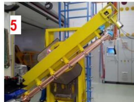
Structure reversed to horizontal position on a temporary girder
