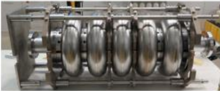
FRIB elliptical cavity assembled with supporting frame
