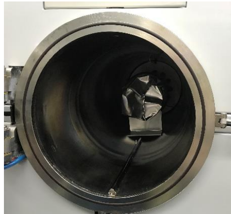
Small furnace for 1-cell. Heater placed in the outer vacuum, very high vacuum (< 2E-7 Pa)
