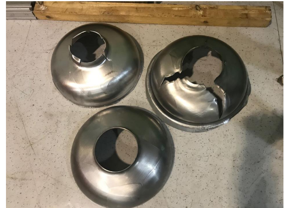
Half-cells broke after deep-drawing
