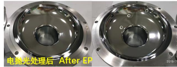
Sample cavity Roughness (Ra) after EP: ~300 nm
