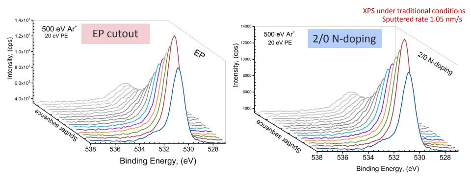
On the removal of surface layers, the concentration of oxygen atoms in the near-surface region decreases, with slight changes in the O 1s spectral profile in the first two sputtering circle. From sputtering circle 3, the O 1s spectral profile for both samples not shown differences.
