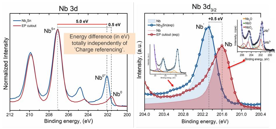
In Nb<sub>3</sub>Sn, Nb atoms have a positive character (compared to metallic Nb); the Sn atoms are subtracting electron density from their Nb neighbors ∴ the interaction of Nb ↔ H, N and O is weaker
