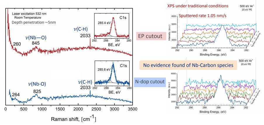
The sorption of the carbon species varies with the chemical composition at the surface layers (Raman spectra) and its presence is limited to the top surface layer (XPS).
