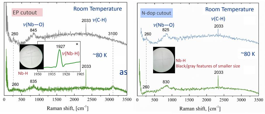
Raman spectra recorded under RT and cryogenic conditions (~77K)
