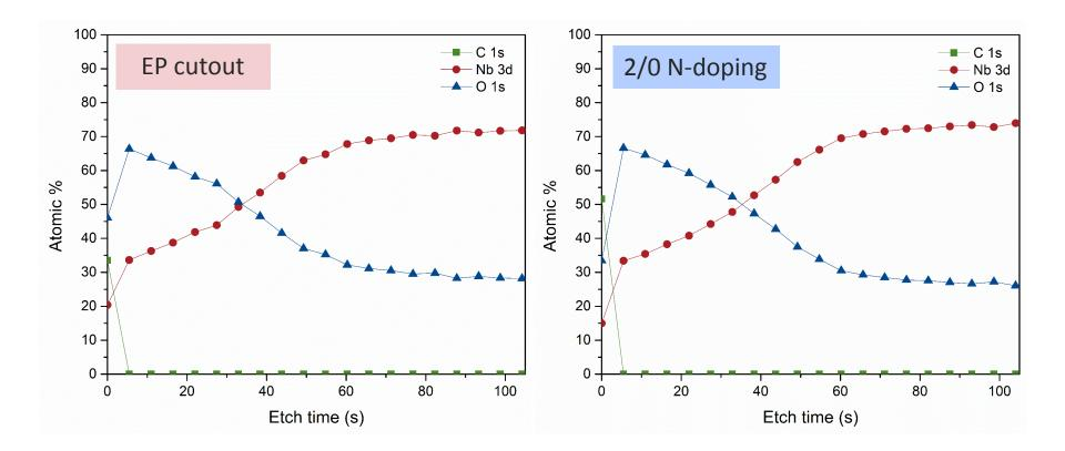
The presence of N atoms could be sensed by the preferential etching in Nb 3d spectral profile favoring the reduction of Nb in Electropolish compared to N-doping cutout cavity.
