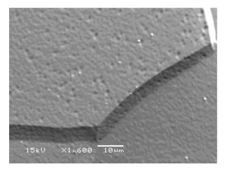
The presence of a large amount of small pores at surface of this cutouts from cell1 suggests that the near-surface region was initially occupied by aggregates of particles of a different nature from the matrix. Such surface porosity, could also be related to a differential attack during the cavity's EP treatment.
