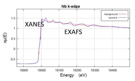
XANES = X-ray Absorption Near-Edge Spectroscopy EXAFS = Extended X-ray Absorption Fine-Structure **Element Specific:** Absorption edges are element-specific
