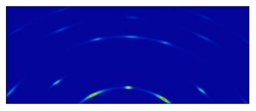
X-ray diffraction, E = 16 keV:  $\Rightarrow$  Polycrystalline, textured foils
