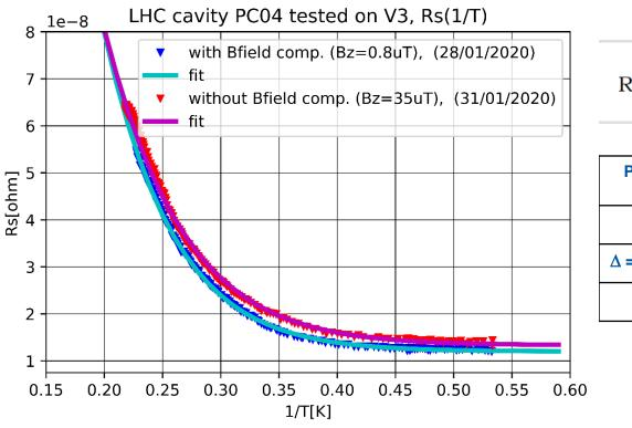
$$R_{s}(T) = A(\lambda,\xi,l,v_{F})\frac{\omega^{2}}{T}exp\left(-\frac{\Delta(0)}{k_{B}T}\right) + R_{res}$$
